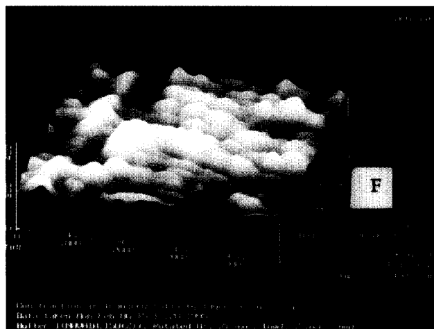
Figure 4 5 \times 5\ \mu\text{m}^2 AFM scan of a transcrystalline layer at 20\ \mu\text{m} radial distance from the surface of a carbon fibre ('F' marks the position of the fibre)
